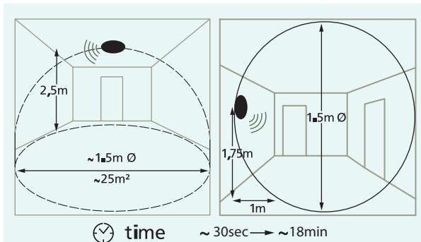
These luminaires are equipped with an integrated motion sensor. The sensor is invisibly mounted behind the glass.
