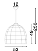
DESTIN - 9586691 Black Rattan Black Fabric Wire & Base LED E27 1x12 Watt 230 Volt IP20 Bulb Excluded D: 53 H1: 49 H2: 250 cm
