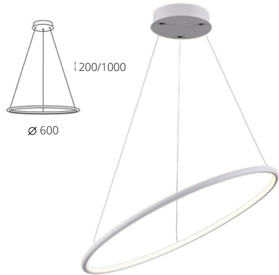
▲ MOD877PL-L36W LED 36W H min: 200, H max: 1000, D: 600 mm, 2300 Lumen, 3000 K, 80 RA, 120 °, 220-240 V, IP20
